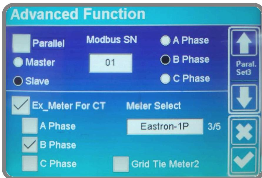
5. Please tick "Ex\_meter For CT" and select the right meter. Choose the corresponding phase if configuring a single-phase inverter. In addition, please select the "slave" option for Modbus and enter the specified Modbus SN.
